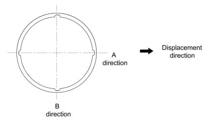
Generally, the displacement direction is referred to as direction A, and the direction perpendicular to it is referred to as direction B, as shown in the figure.
