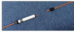
③ Connect the wire by soldering and cover with the insulating tube for insulation.
