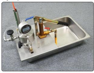
The digital hydraulic calibrator set is a self-calibrator (model HC-15S) for testing or calibrating a vibrating wire piezometer. It combines a hand pump set with a piezometer clamp that is made differently by model. Calibration by using digital pressure gauge and water pressure makes easy and accurate calibration possible. The calibrator set is mostly made of stainless steel.
